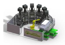
Molding plant made of 6 machines served by anthropoid robot
